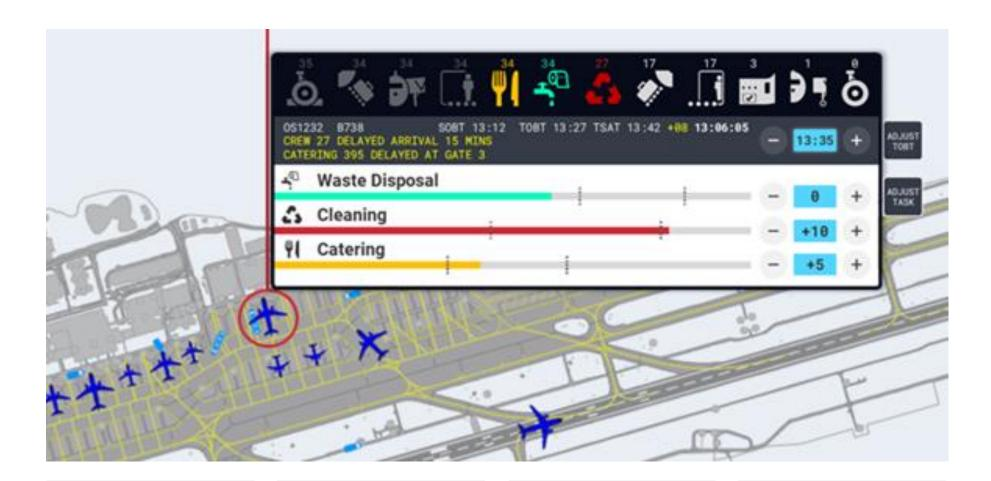
Symbolize aircraft movements with scheduled, estimated and actual A-CDM timestamps Display turnaround process and progress based on aircraft type and task time tables
