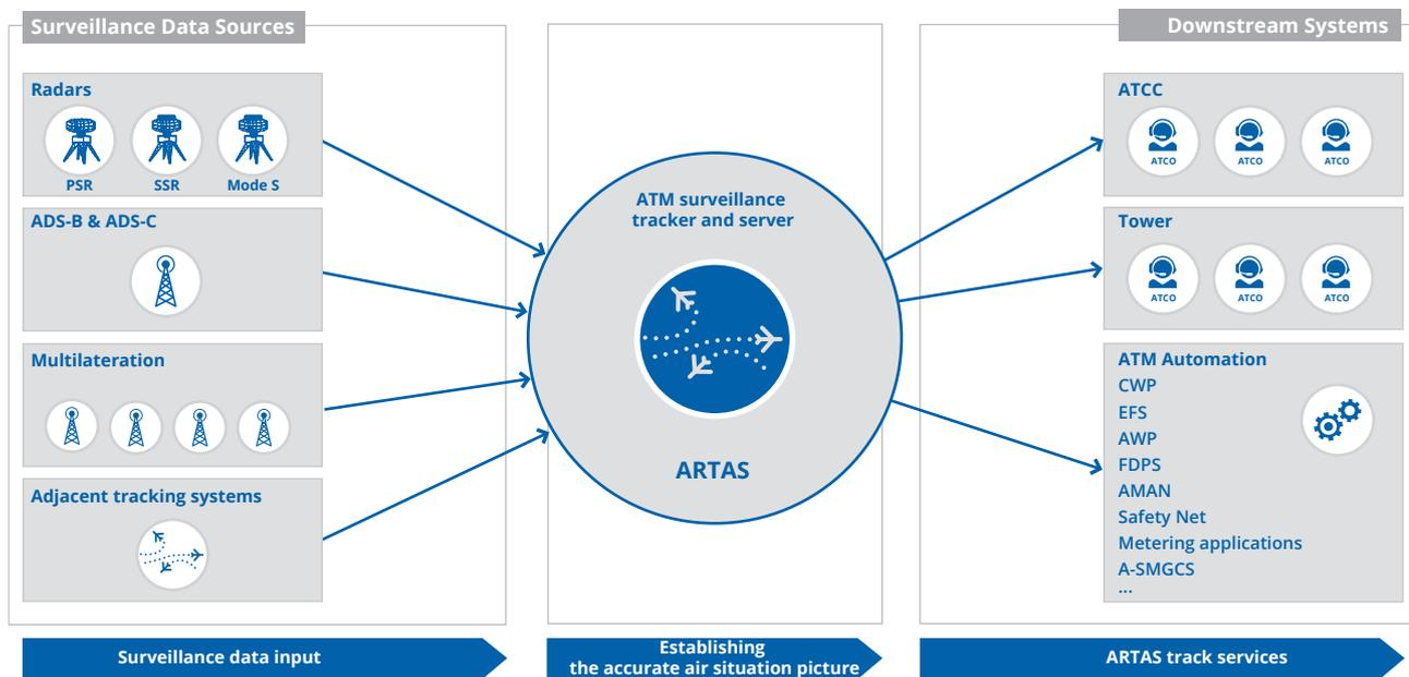
Figure 2: Schematic of ARTAS inputs and outputs
