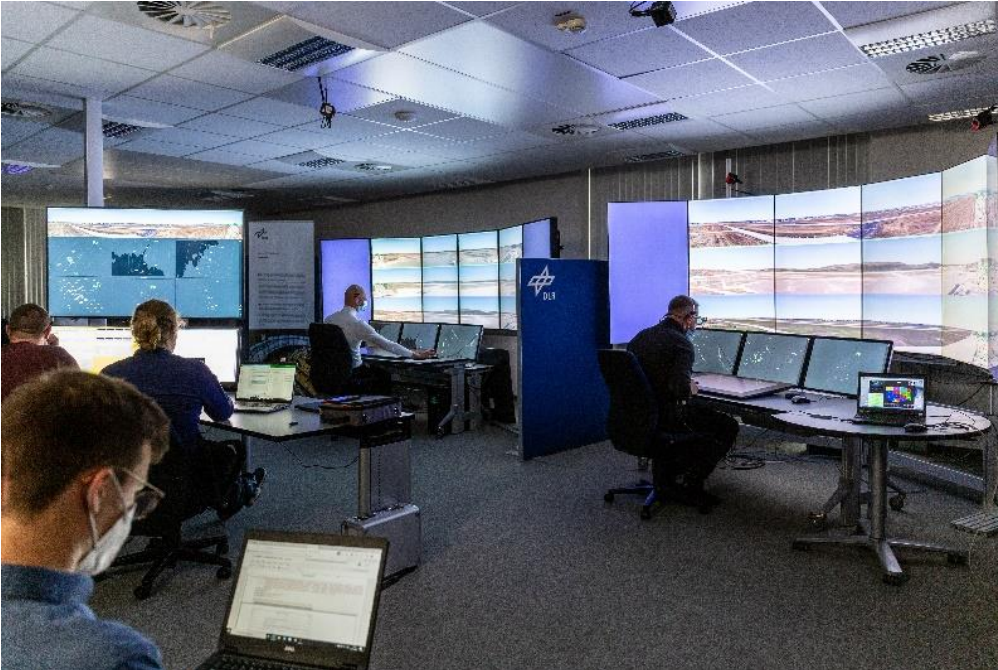
A Remote Tower Centre prototype was set up to control 15 simulated airports as realistically as possible from a remote location. © DLR
