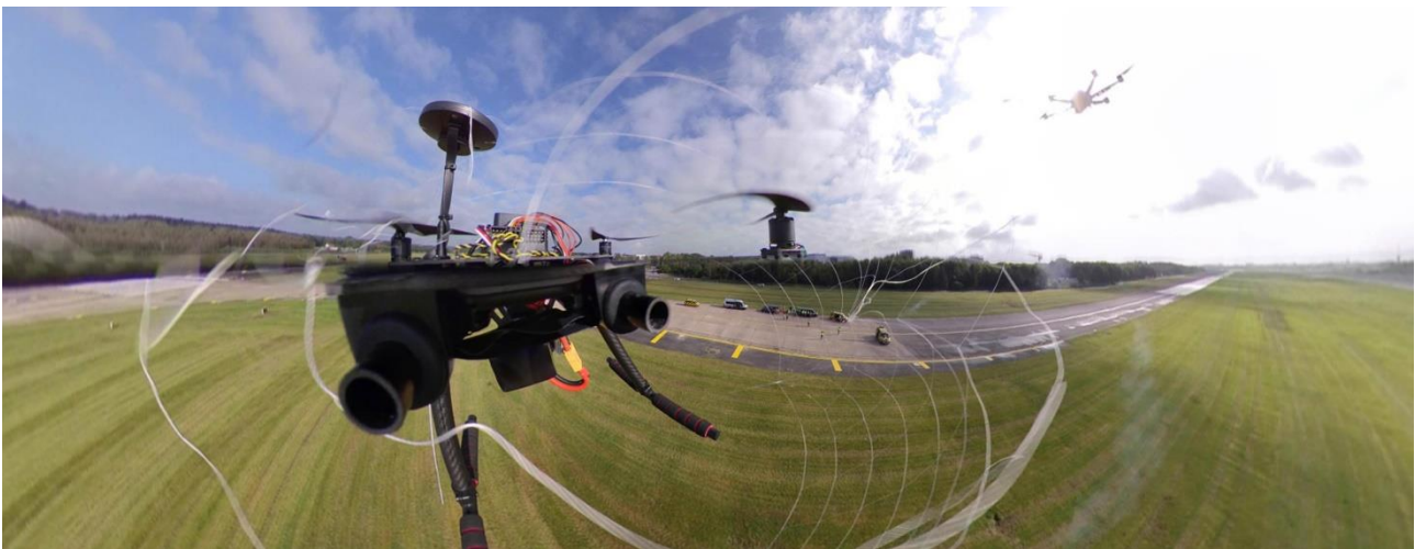
Non-cooperative drone being caught with a safety net during flight (© Frequentis)
