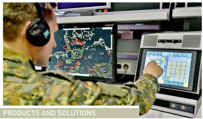
iSecCOM is a highly available distributed IP voice communication system which supports integration of voice encryption devices and provides domain separation via a secure audio switch.
