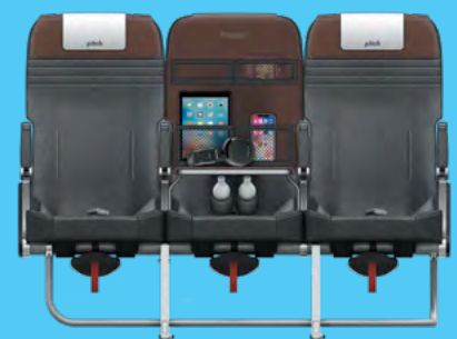
Console yourself: Pitch Aircraft Seating’s Q Premium concept for single-aisle fleets.
